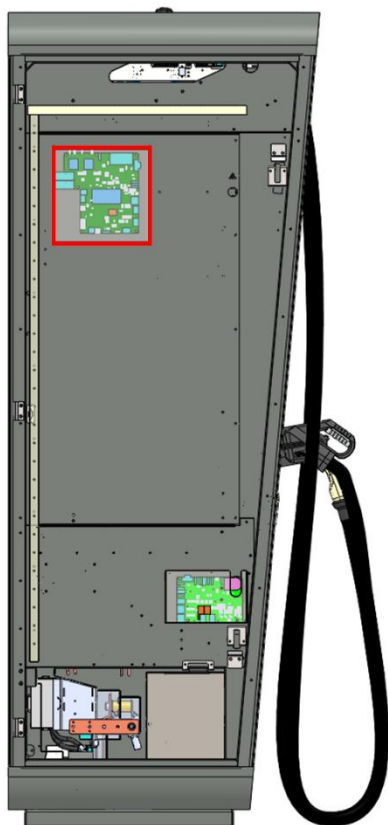
Figure 30: Position of the CTRL_COM in the Hypercharger
