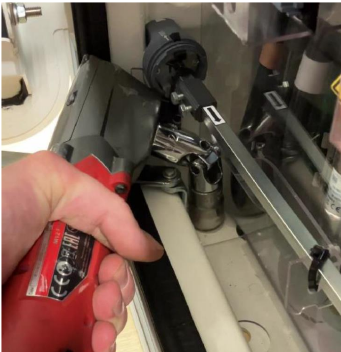
Figure 43: Angle adapter insert for pallet screw removal
